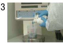
Check and mix colour using 3MTM Paint Preparation System. Spray a test panel, assess and confirm the colour match and coverage using the 3MTM PPSTM Colour Check Light (16407).
