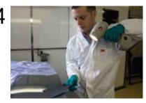
Compare variant Colour Cards to the vehicle being repaired and choose the colour card that best represents the actual vehicle colour using the 3MTM PPSTM Colour Check Light (16407).
