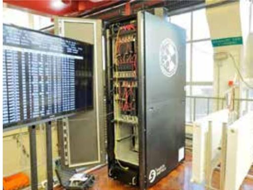
The Iceotope system has a monitored power use of 2.3kW. Approximately 100W is required to reject the heat from the system into the laboratory via the radiators. If a similar air-cooled system were installed in Leeds' existing HPC data center it would require 885W of air-based cooling. This represents a more than 80% saving on cooling energy consumption, according to project organizers.
