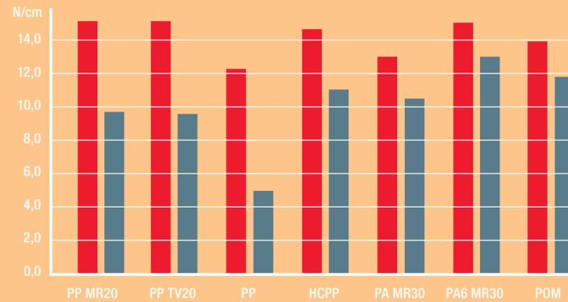
2. Peeling resistance on various surface textures (peak-to-valley depth in  $\mu\text{m}$ )
