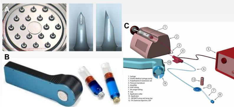
A) Hollow microneedle array (hMTS); B) hMTS injector and cartridges filled with methylene blue solution ; C) Quick Evaluation Device for controllable delivery of liquid formulation.
