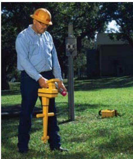
The 3M™ Dynatel™ 2200 Series Locator is used to program as well as locate buried markers such as those buried with the SASD force main pipelines. Information programmed into each ball can be read remotely on the locator screen.
