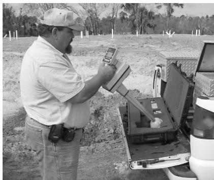
Ron Witt, Charlotte County Utility Field Inspector, programs a marker ball. Stored information includes pipe type and size, the year of installation, fitting type, and depth below the surface.
