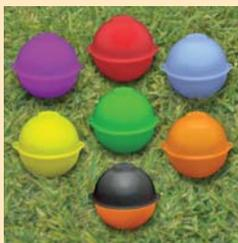
*The four-inch ball markers used by Southwest Gas can be located using a 3M 1264 EMS II Marker Locator or a 3M Dynatel 2200 Series Locator. Distinctive marker colors and operating frequencies are assigned for each utility in accordance with American Public Works Association standards.*
