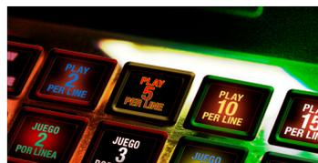
Figure 3: OLED Buttons (dynamic content/fixed location)
