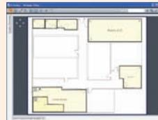
The CAD system includes a facility to map the network on drawings of the building layout allowing an 'at a glance' view down to outlet level.
