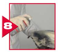
If necessary 3M™ Automix™ Superfast Plastic Adhesive 55045 can be painted using usual paint process for plastic parts or specific bumper paint in spray.
