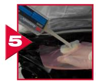
Cut 3M<sup>™</sup> Contour Sheet 04903 to about 2.5 times the size of the tab to be repaired. Apply 3M<sup>™</sup> Automix<sup>™</sup> Superfast Plastic Adhesive 55045 with 3M<sup>™</sup> Applicator 08190 using the Contour Sheet as support.
