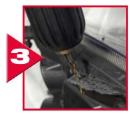
Drill several holes of 3-6mm in diameter in the remaining part of the tab to increase the strength of repair.
