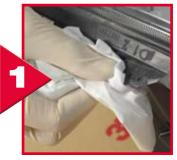
Apply 3M™ VHB™ Surface Cleaner or 3M™ General Purpose Adhesive Cleaner 08984 using 3M™ Professional Panel Wipe 34567 to clean the area. Allow to dry completely.
