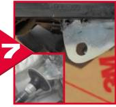
After 5 minutes shape tab using a 3M™ Roloc Disc P80/180 and create a new fixing point to restore original appearance.
