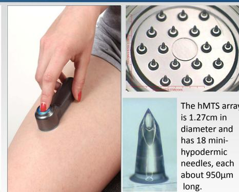
The hMTS array is 1.27cm in diameter and has 18 mini-hypodermic needles, each about 950μm long.
