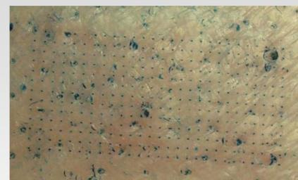
Methylene blue was used to stain swine skin (in-vivo) following hand application of the MSS device with < 2lbf. Each blue spot corresponds to a microchannel created in the stratum corneum.
