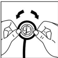
With the diaphragm side up, grasp the rim with the thumbs and index fingers of both hands and roll the rim off the edge of the chestpiece.
