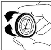
Visually examine the ring to ensure that the flexible edge is smoothly engaged inside the rim. If necessary, flex the assembly by pinching the outer rim edge between the thumb and fingers. Repeat this
