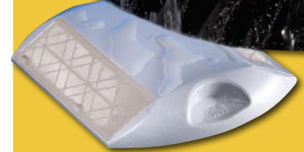
The Series 290 stud gives maximum impact resistance. When tested according to ASTM standards, the marker body displays no cracking or breakage using a 1000 gm weight from a height of 1 metre.
