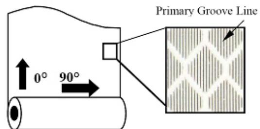
Figure 1 – Sheeting is positioned at 0° application angle.
