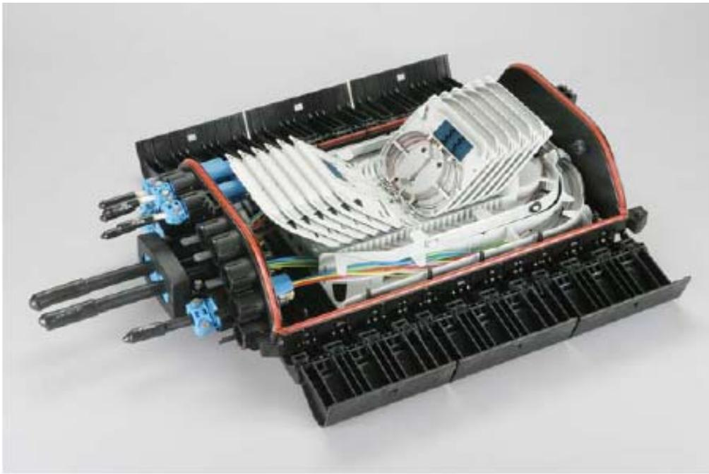
Watertight splice closure for up to 168 mechanical Fibrlok splices or 336 fusion splices (BPEO size 2)
