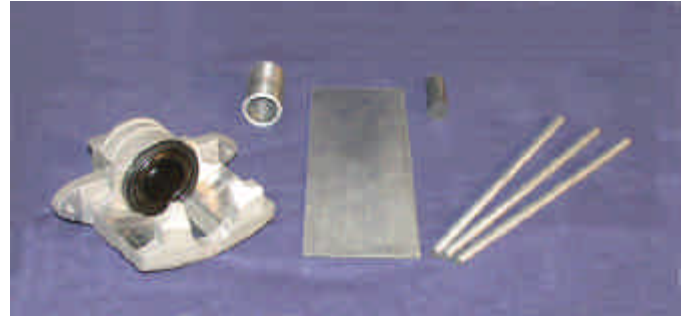
Traditional casting technology produces metal matrix composites in nearly any geometry.
