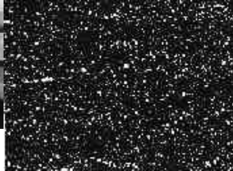
Typical fiber distribution in CFAMC.
