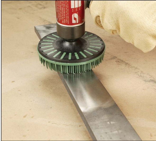
4.5" bristle disc (grade 50) cleaning mill scale
