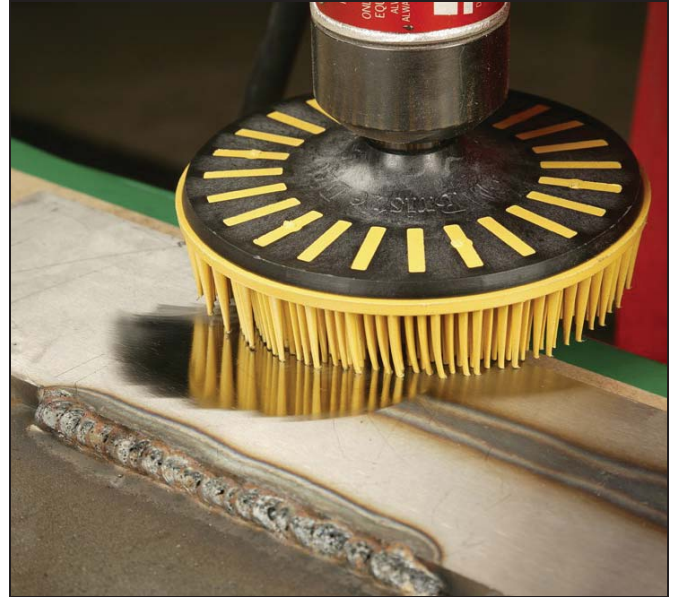
4.5" bristle disc (grade 80) removing weld burn
